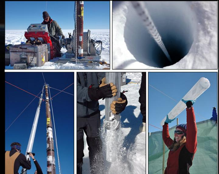
Drilling of ice cores to obtain  $^{10}\text{Be}$  measurements
