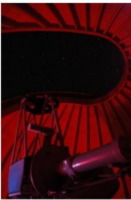
The 65 cm reflector, equipped with a photometer, is used mostly for the study of the <u>variable</u> stars
