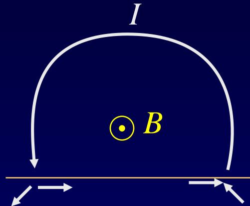
$$\left. \begin{array}{l} \Phi = L I \\ \Phi \approx \text{const.} \end{array} \right\} \Rightarrow \left. \begin{array}{l} I \propto L^{-1} \\ L \propto R \end{array} \right\} \Rightarrow \begin{array}{l} \Delta I / \Delta R < 0, \\ \Rightarrow \Delta F_L / \Delta R < 0 \\ \Rightarrow \Delta W / \Delta R < 0 \end{array}$$
