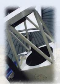
diameter of 400 mm (focal ratio of f/6.8), and the other one with a diameter of 260 mm (focal ratio of f/15). The telescope pointing and tracking are controlled by the computer. ACT is equipped with CCD camera and mostly used for observations of open clusters and variable stars.
