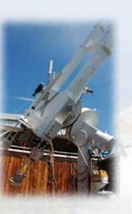
It provides valuable data for studies of rapid changes of chromospheric and photospheric features in great detail. Using a field of view of about 7 and 11 arcmin, its aim is to produce the high-resolution images of active regions on the Sun to complement patrol full-disc images.
